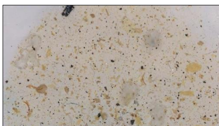
Microscope image of microplastic fragments isolated from farm soil.
