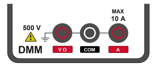
This typical multimeter terminal panel is rated for measurement connection up to 500 V with respect to earth.
