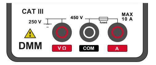
This multimeter is rated for mains measurement connection up to CAT III 250 V with respect to earth and 450 V between terminals.
