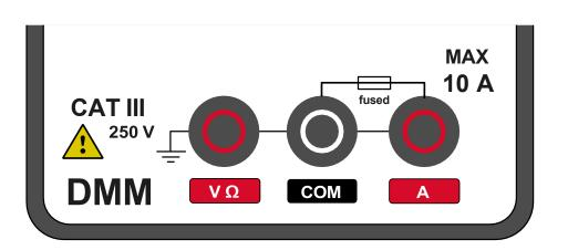
This multimeter is rated for mains measurement connection up to CAT III 250 V with respect to earth.
