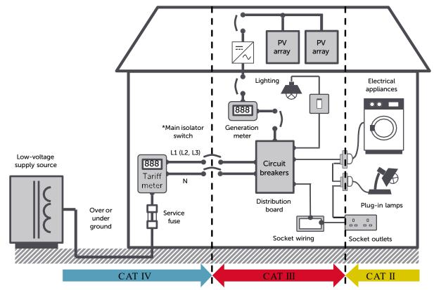
Footnote: In some installations the main isolator switch may be the device provided by the DNO. Where this is not the case it will be on the distribution
