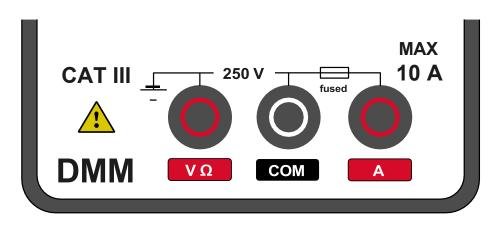
This multimeter is rated for mains measurement connection up to CAT III 250 V with respect to earth and 250 V between terminals.
